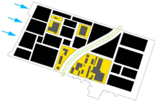
3 ADJUSTMENT OF GRID TO AVOID WIND TUNNELS GRID'ET JUSTERES FOR AT UNDGÅ VINDTUNNELLER
